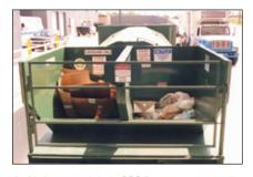
At this large hospital, the DRC II averages 60% trash in one compartment and 40% cardboard in the other compartment. This provides convenience and flexibility with only one unit.
