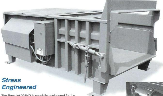
The Ram-Jet 225HD is specially engineered for the really tough jobs in waste disposal, and that means the strength is where it belongs... charge box floor features 1/2" steel plate over four 4" steel channels... 1/2" ram face plate, backed with 10" channels that incorporates T-1 plate in high stress areas... 3/8" ram top supported by 8 heavy duty formed crossmembers... and heavily reinforced charge box sides.
