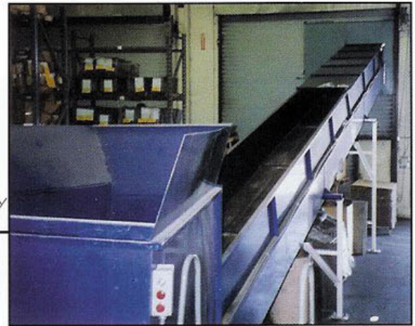
This thru-the-wall sliderbed conveyor application feeds a compactor on the outside.
